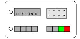
**5. Monitor Status LEDs throughout the process:** At beginning of EQ, the AC2 In Good light should flash. At the end, the Float light will light up. Equalizing can take 2 to 6 hours, typically.
