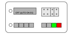
**4. ENGAGE EQ MODE:** Press the <u>Green</u> button to go to the Generator Mode menu. Press the <u>Set Point</u> right or left button to move the underline under EQ. If you have two or more inverters, repeat this step on all inverters.
